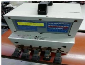
5 Spindles Automatic Coil Winding Machine
