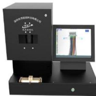
Wire Color Sequence Testing Instrument
