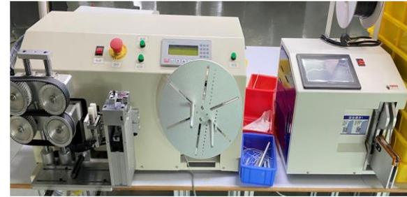
Automatic Cutting and Winding Machine
